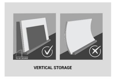
The exposed sheet should be covered, and the edges secured from any accidental damage. A heavy board can be used at the free end to prevent slippage and damage.
