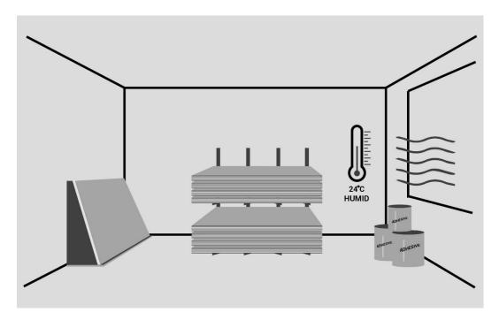
The conditions can vary depending on general environmental conditions in the geographical area. In case of a significant difference in ambient conditions, preconditioning time ranges from 5-7 days.
