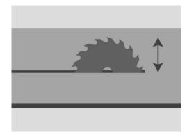
If the uppercut edge quality reduces, the saw blade can be set higher. The saw blade should be set lower in case of an unclean cut to the bottom. The best height setting should be judged appropriately. Saw entry angle of 45° is considered as optimal. To achieve this, maximum 10 percent of the saw blade diameter should protrude over the workpiece.
